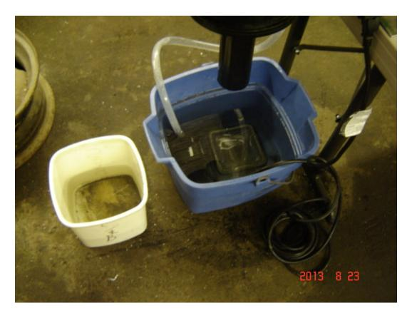
Place large bucket with block water pump and hose as shown. Put small bucket on top of block.
